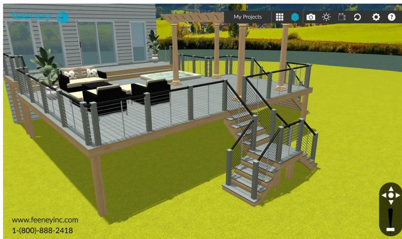
Decks can be viewed in either 2D or 3D representations, and intuitive features such as click-and-drag sizing tools and “smart” icons make it easy to change dimensions, add stairs and additional tiers, and modify the shape of the deck. Users can choose from a variety of deck materials and add walls, windows and doors to replicate the facade of a home or commercial building.
