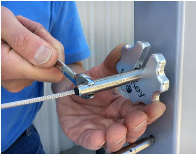
Manufactured from lightweight and durable 6061 aluminum alloy for long-lasting performance, the Quick-Connect® Wrench Wheel allows for continuous full rotation without requiring repositioning of wrenches – making it a faster and easier alternative to the two-wrench tensioning method. The tool utilizes a specially designed spring ball retainer that securely grips onto the wrench flats of the Quick-Connect® Tensioner fittings for ease of maneuvering.
